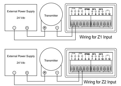
For three or four wire transmitters follow the wiring instructions provided with your transmitter.
